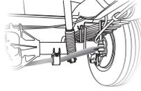
**STANDARD FRONT STABILIZER BAR** Reduces the body roll of a vehicle during cornering or over road irregularities
