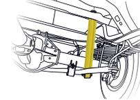
**KONIG® SHOCK ABSORBERS** Controls bounce and sway when driving over expansion joints and rough roads
