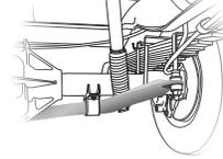
**HEAVY-DUTY REAR STABILIZER BAR** A larger bar and polyurethane bushings, instead of rubber, transfer power faster for extra support, more stability and easier handling
